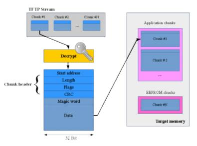
Fig. 3: Uploading chunks mechanism.
