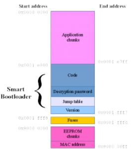
MAC address dx8000 00tf Fig. 1: The whole address region of Netzer with all address positions of the bootloader and the installable application.
