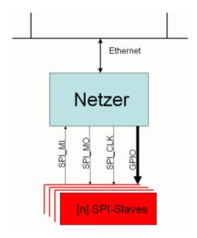
In contrast to the base version the pro version uses no dedicated chip select signal. But there exist special escape sequencies for accessing all the pins of Netzer which are configured as digital outputs. Thereby up to 10 different slaves can be selected. Also other control pins can be serviced which are sometimes needed by special SPI modules. All Netzer GPIO pins but SPI\_CLK, SPI\_MO and SPI MI are free usable and controllable via the web interface or the GPIO server.
