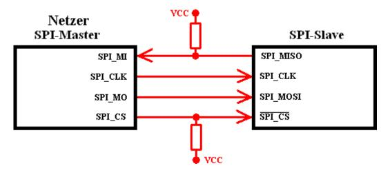
The SPI\_CS shall be low active - a low level selects the slave. The pull up resistor at CS is needed to prevent false selection. This may occur on power up if CS is not driven by Netzer. The pull up resistor at SPI\_MI is needed to prevent floating in case the slave is not selected and therefore the pin is not driven.
