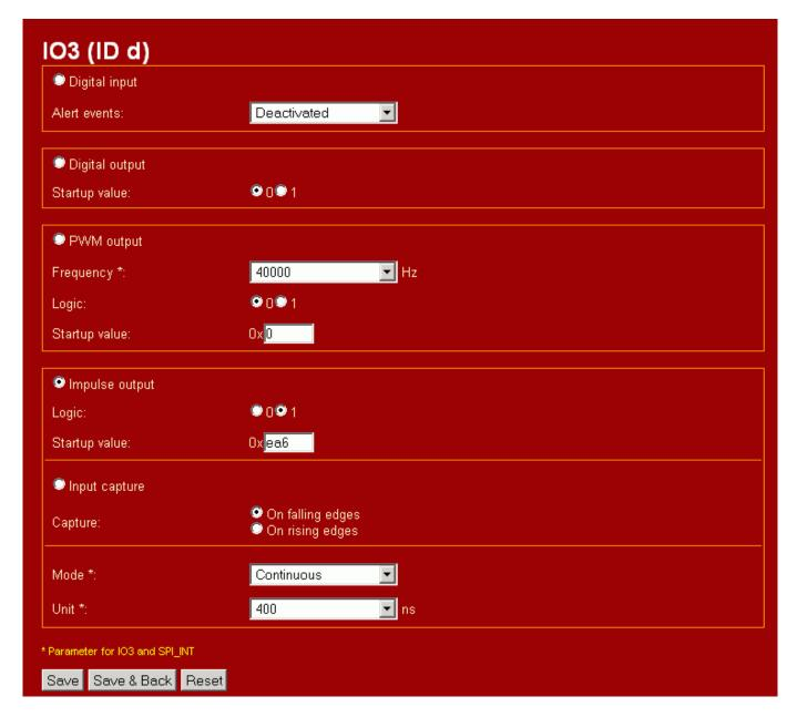
The periodic time results from the internal 16-bit counter for continuous pulse signals: 65536 \* 400 ns = 26,21 ms.
