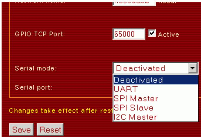
The interface as well as the TCP/IP-port of the serial server are set on the website with the general settings. The new settings always become only active after restart of the Netzer.
