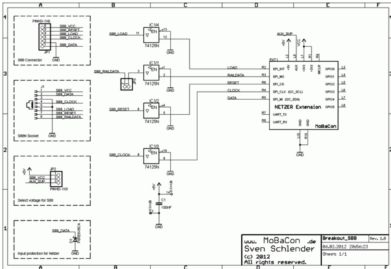
The picture shows a circuit for the Netzer [Playground](#) S88 Extension board. The used parts are standard components, which can be build up fast also on a grid-style board.
