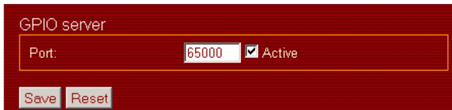
For simple tests of the server and the protocol every terminal program may be used that is capable of building up connections via Raw TCP sockets, such as e.g. the Windows HyperTerminal.
