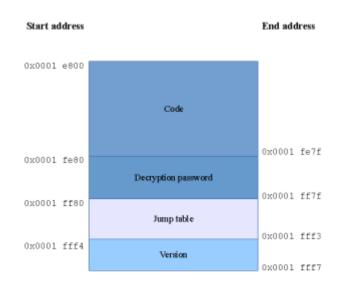
Fig. 2: The detailed structure of the bootloader and its addresses.
