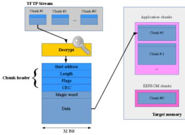
In figure 3 such a TFTP stream is shown, as they arrive in the bootloader. In the stream there can be a lot of small chunks. The chunks are decrypted (if decryption is enabled) on the fly.
