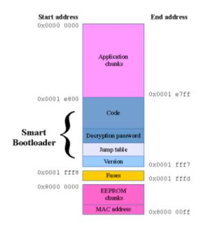
Fig. 1: The whole address region of Netzer with all address positions of the bootloader and the installable application.
