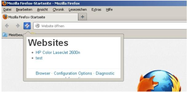
Comfortable Netzer discovery is possible with Firefox browsers and the installed DNSSD-Plugin. This plugin maintains all found web pages of MDNS devices in a list. Netzer has a name like *nexxyyzz.local*. *xxyyzz* are the last three numbers of its MAC address. The name can later be changed on the Netzer web sites.
