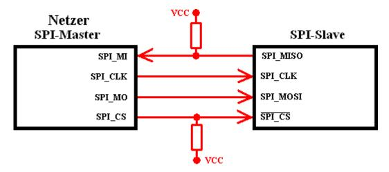
The SPI\_CS shall be low active - a low level selects the slave. The pull up resistor at CS is needed to prevent false selection. This may occur on power up if CS is not driven by Netzer. The pull up resistor at SPI\_MI is needed to prevent floating in case the slave is not selected and therefore the pin is not driven.
