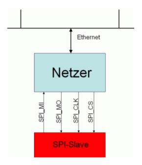
With the free downloadable base version exactly one slave is supported. Also chaining of more slaves is supported because therefore only vxcyone chip select is needed. The example circuit like the figure above consists of the four pins SPI\_MI, SPI\_MO, SPI\_CLK and SPI\_CS. SPI\_MO is the data output (data from Netzer to slave). SPI\_MI ist the data input (data from Slave to Netzer). The clock signal (SPI\_CLK) is controlled by Netzer.
