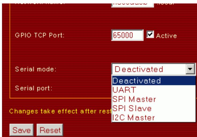
The interface as well as the TCP/IP-port of the serial server are set on the website with the general settings. The new settings always become only active after restart of the Netzer.
