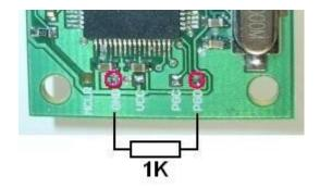
The PGD pad should be pulled down with a resistor (1K) to ground during a Netzer restart.
