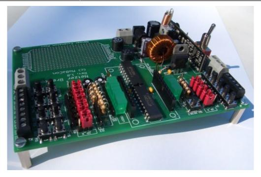
The module has the dimensions 134  $mm \ge 90 mm$ . All delivered parts are THT parts. The level for assembly is estimated as medium difficult, because of the amount of parts to assemble.
