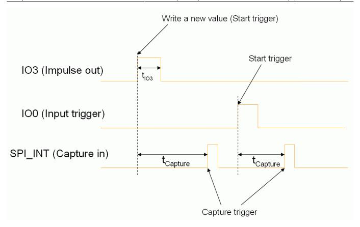
The second example shows the special case of an ultrasonic sensor like HC-SR04. This sensor needs a 10 µs impulse at the TRIG input which shall be connected to IO3. The pulse length of sensor singnal ECHO decodes the distance to the detected object. The signal must be connected to IO0 and SPI\_INT. IO0 must be configured for rising trigger edge, SPI\_INT for falling capture edge.
