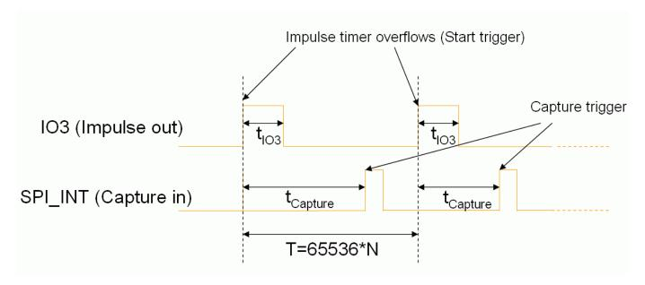
Measuring impulses in single mode (Unsynchronized)
